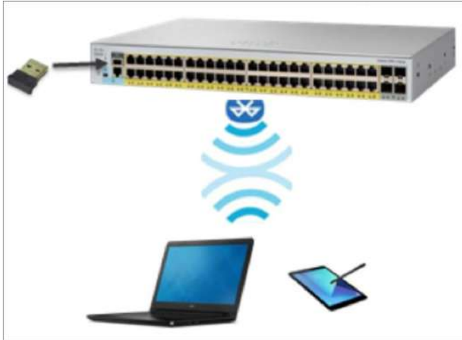
Figure 2. Over-the-air switch access using Bluetooth
