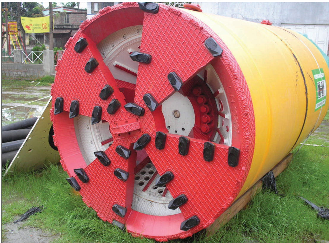
Micro Tunneling Machine
